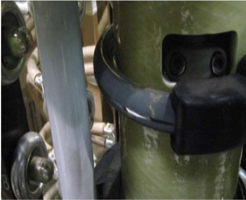
AgS on OLTC contacts and collector rings
