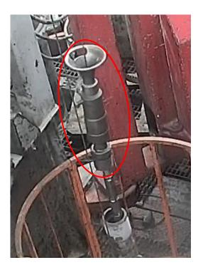
The drilling and wireline team was in the process of removing a dummy drift from the recovery tube after a downhole run. As the wireline equipment was being retrieved, it became disconnected from the tool, causing the gland packer to fall from a height narrowly missing a worker.
