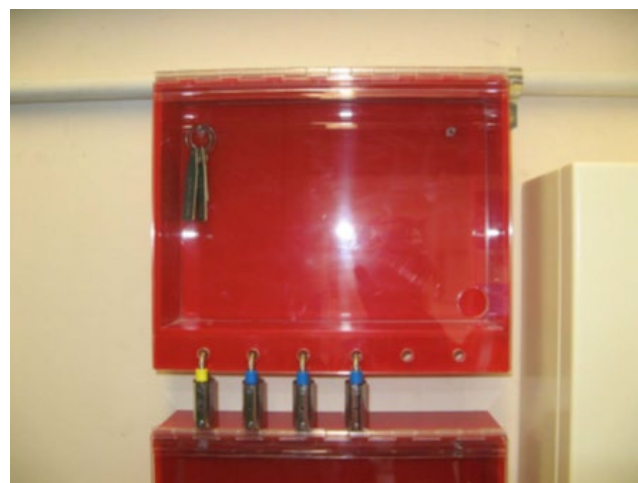
Picture 1: Example of lock box
