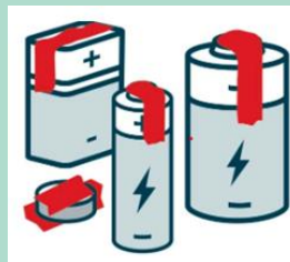
Batteries taped correctly
