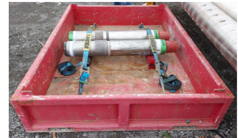
Secured to cradle within a basket
