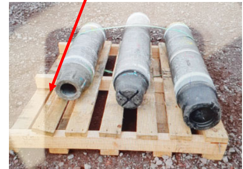
Lifted pallet rung releasing tension
