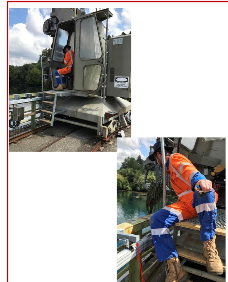
Simulation of sitting position whilst sitting on step and fence bracket which impacts below the right knee
