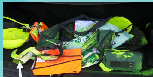
Bottom of aerosol can blown off
