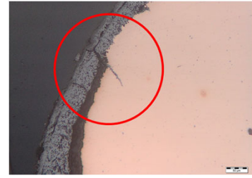
Pitting/crevice on copper wire due to corrosion
