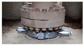
These clamps serve to hold compressive force against well pressure and will retain the bull plug in the event of a failure.
