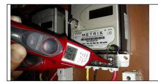
Photo demonstrates voltage present on load side when meter line side had been isolated.
