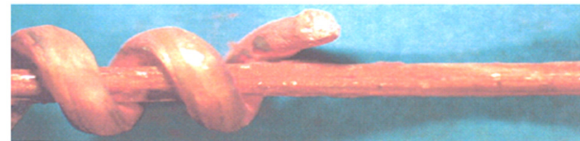
(c) Wire Break - Fail
